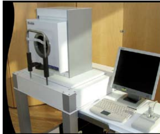
Figure 22-2. The Preciso topographer/tomographer uses Scheimpflug imaging technology.
